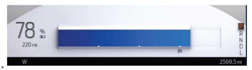
□ Check charge port and charge status indicator function. To open the charge port door, press the center right edge of the charge port door and then release. When the charge coupler is connected to the vehicle, the indicator light will illuminate, and indicate the SoC as shown in Figure below. If the charge status indicator does not light up or pulse after plugging the vehicle in, verify that the charge port light setting in the center stack is set to "On".
